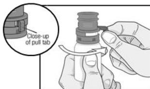
Step 3: Remove the olive green colored protective cap by pulling it straight up. Keep the colored protective cap.
