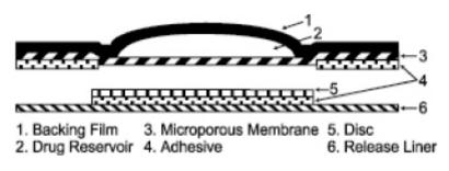
Figure 1: System Schematic
